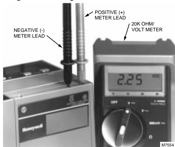
Fig. 20—Flame signal measurement.
